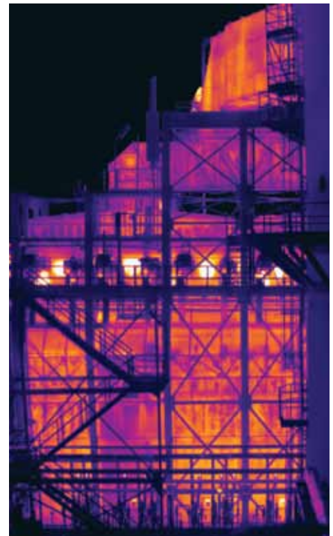
A cabin furnace as seen from a distance of about 80 meters using the FLIR P640 thermal imaging camera.
