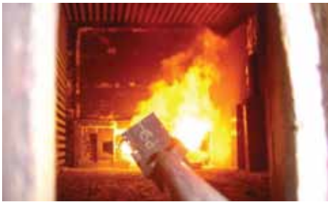
The thermocouple probe is inserted in the furnace. Tournieux then uses the temperature reading to accurately correct the thermal imaging camera for emissivity.
